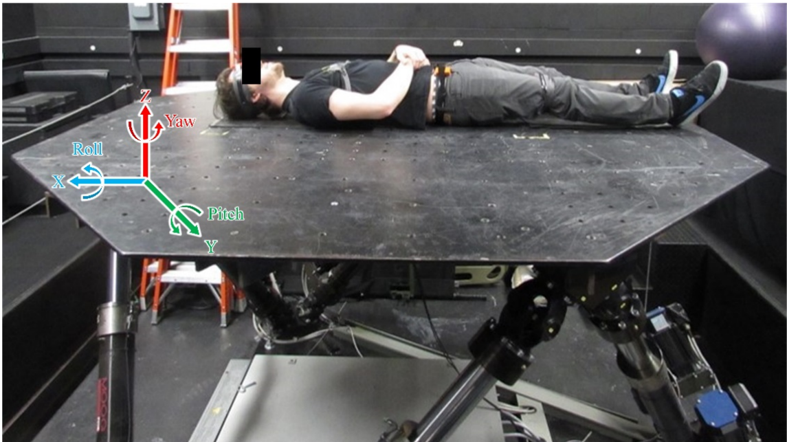
Figure (4.1) Profiles of the supine human testing: the human subject lay on the rigid platform of the motion simulator, and vibrations were generated in the vertical Z direction
